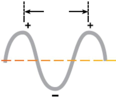
Radio waves oscillate, or flip back and forth, between plus and minus at a predictable rate.
