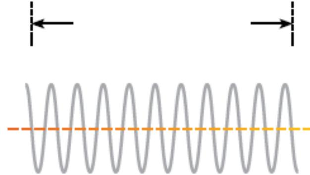
The number of cycles in one second gives the frequency. How “frequently” the signal oscillates in one second.
