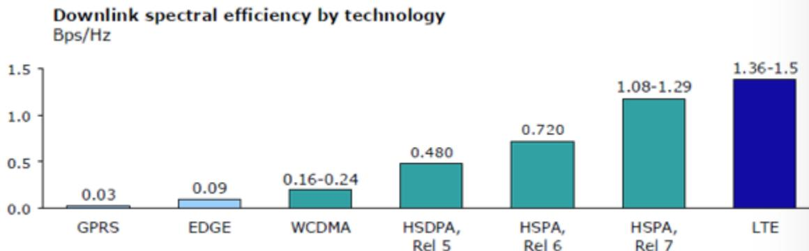
Spectrum Efficiency in Bps/Hz
